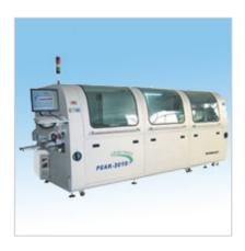
Series: Lead-Free Wave Soldering System
